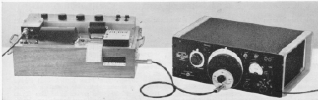
Figure 1. View of the General Radio Beat-Frequency Audio Generator coupled to the Bruel and Kjaer Model BL-2304 Level Recorder by means of the new coupler and flexible cable.
