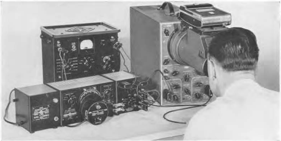
Figure 11. A setup for observing and recording the response of the octave-band analyzer on a DuMont Cathode-Ray Oscillograph. The Type 1210-B Unit R-C Oscillator, which is driven by the 908-P2 Dial Drive, supplies the signal to the analyzer, and the Type 1210-P1 Detector and Discriminator, shown attached to the oscillator, supplies the deflecting voltages to the oscillograph.
