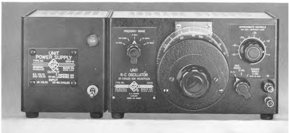
Figure 1. Panel view of the Type 1210-B Unit R-C Oscillator and the Type 1203-A Power Supply. The oscillator plugs into the power supply and can be secured to it with a bolt and butterfly nut to form a rigid assembly.
